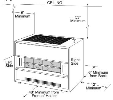
Figure 3 - Heater Clearances
